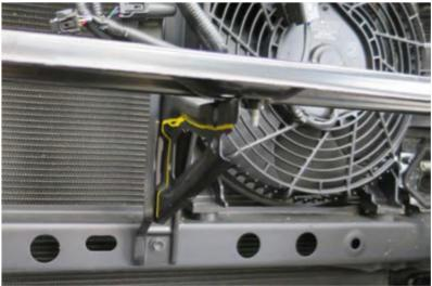
6) You can now remove all wiring & water harness from the original plastic bumper, when removing the sensors make sure you mark them which way is correct up and down and which side is which.
