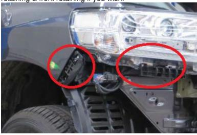
4) Fit mounting hardware, The spacer brackets first then the cradle. The spacer brackets can be tight but keep cradle loose incase you need to move left or right
