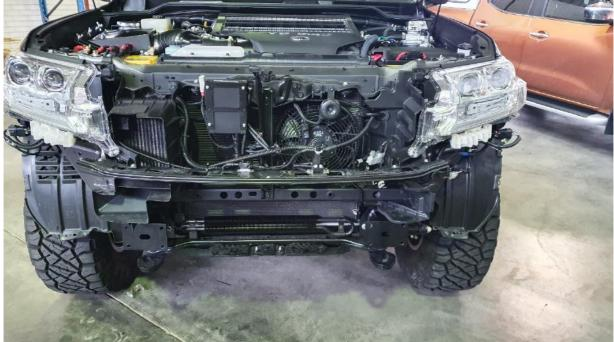
3) Remove grill, front bumper bar, bumper reinforcement and lower bumper support brackets. Also remove bumper retaining clips on side guard, and below headlight as indicated including the plastic side bumper retaining & front retaining if you wish.
